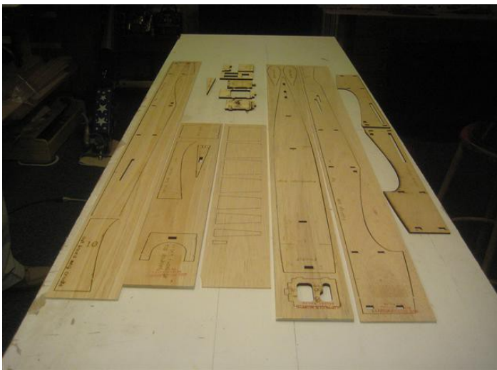
The balsa laser cut parts are still within the sheet stock.
